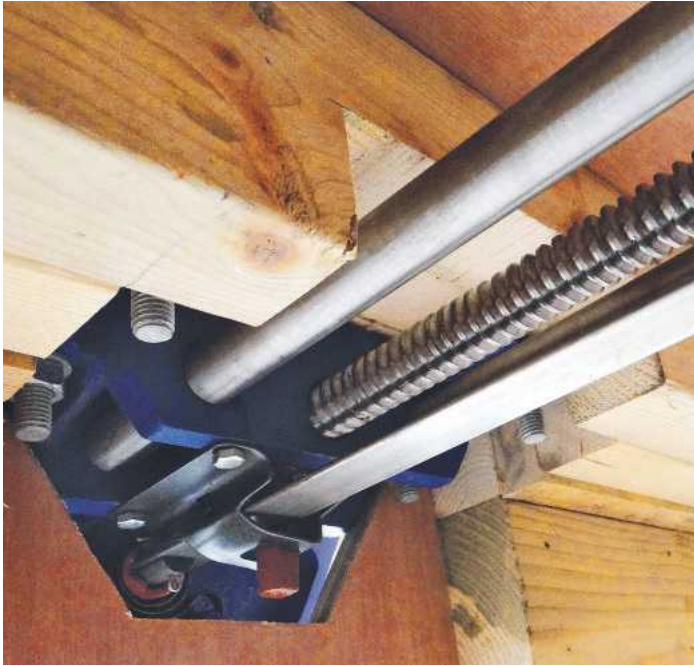
▲ Pic.9 I was lucky; an 18mm fascia meant that the front bolts only just squeaked in. I used some hefty galvanised bolts left over from the log shed, and they worked a treat
